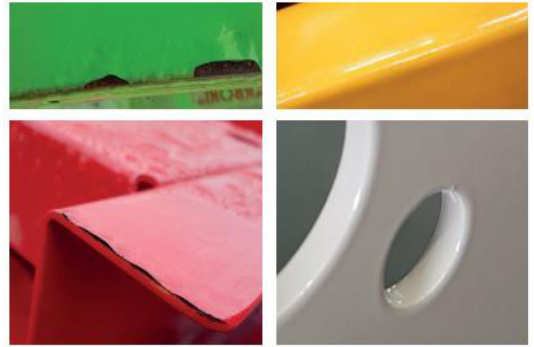
Above: Examples of premature corrosion failure
